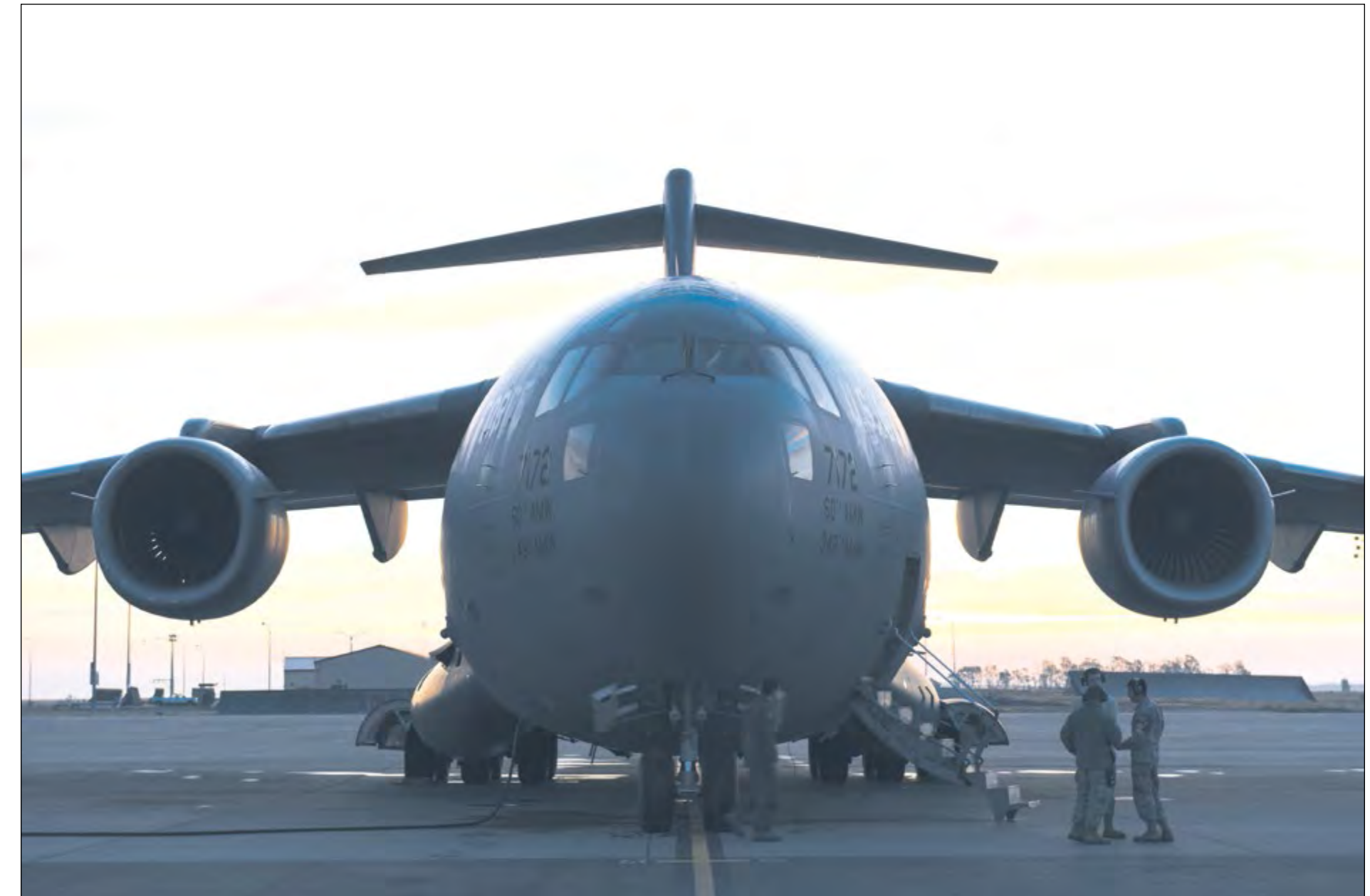
1) A C-17 Globemaster III gets an early morning start on the flight line Oct. 24, 2018, at Travis Air Force Base, Calif. A C-17 has a maximum takeoff weight of 585,000 pounds and a wingspan of more than 169 feet.
